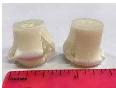
Figure 23. ABS Specimens of Sparse Structure Printed by Fortus at flat-90° Print Orientation After Compression Test.
