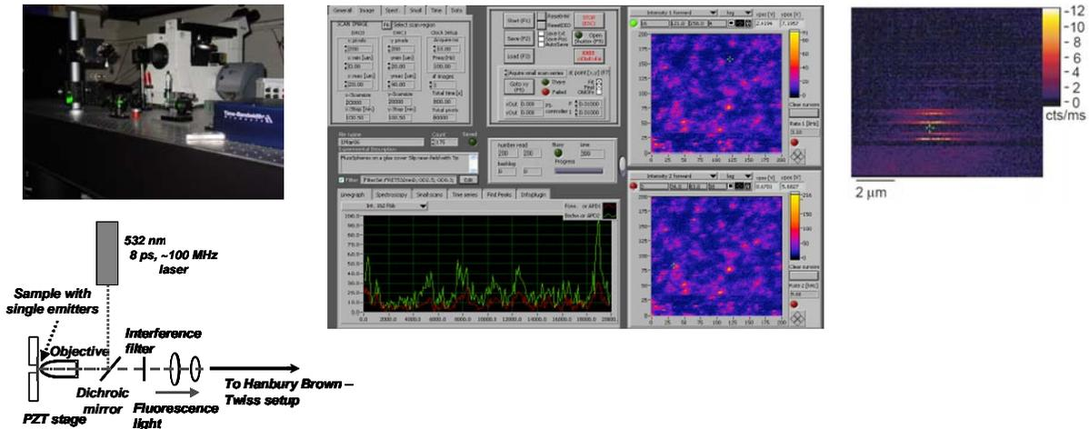
Figure 3. Left: Photograph and schematic of a home-built confocal microscope; center: user interface for single-emitter fluorescence imaging. Images of a raster scan of the sample show DiI-dye single-molecule fluorescence; right - single PbSe quantum dot fluorescence image in 1-D photonic bandgap liquid crystal host (800 nm fluorescence maximum).
