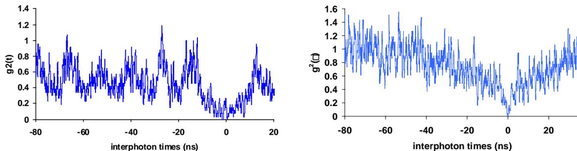
Figure 5. Left: fluorescence antibunching of single PbSe quantum dot on bare glass slip under pulsed laser excitation; right: fluorescence antibunching of single CdSeTe quantum dot in 1-D photonic bandgap cholesteric liquid crystal host (fluorescence lifetime of quantum dots is higher than the time interval between laser pulses).
