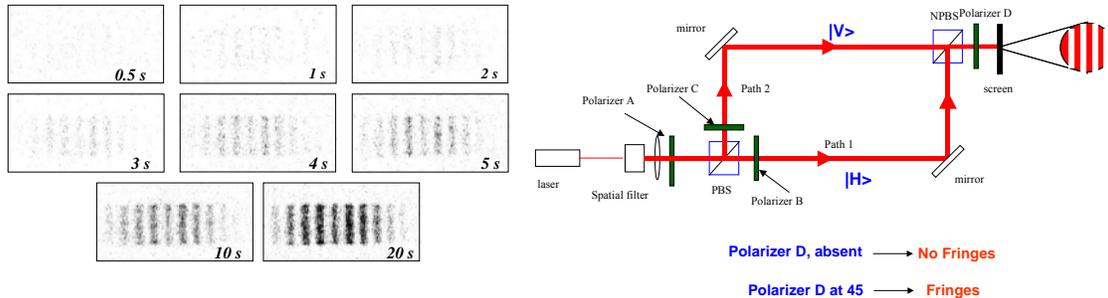
Figure 2, Left: single-photon interference using Young's double-slit at different exposure time. Right: Mach-Zehnder interferometer schematics for "which-way experiment".
