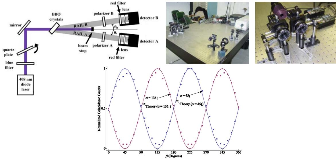
Figure 1. Top left: schematics of entanglement and Bell’s inequalities experiment with a blue diode laser; top right: photographs of entanglement lab setup and entangled photon registration module of an argon ion laser setup; bottom: experimental polarization correlations.
