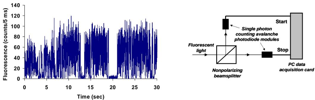
Figure 4. Left: changes of fluorescence intensity of single CdSeTe quantum dot in time (blinking); right: schematics of a Hanbury Brown and Twiss setup for fluorescence antibunching measurements,
